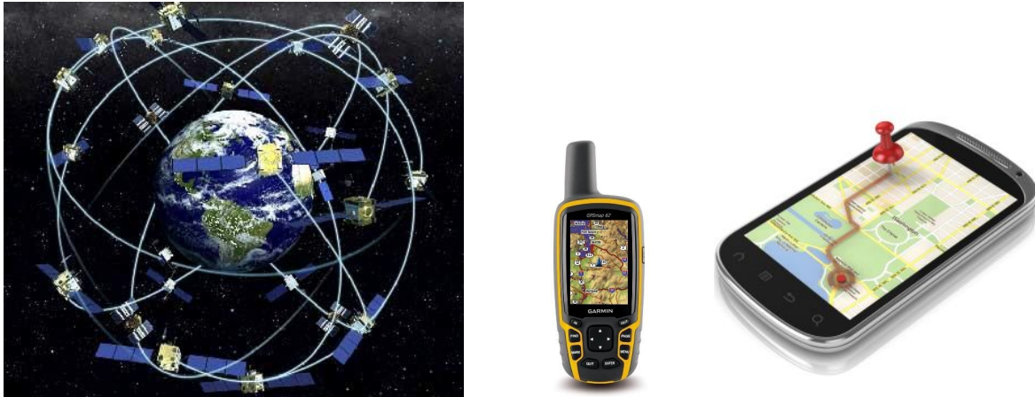
Figure 3.1: (left) A diagram of the satellite-based GPS system, (right) examples of devices that can receive transmissions for the GPS satellites.
