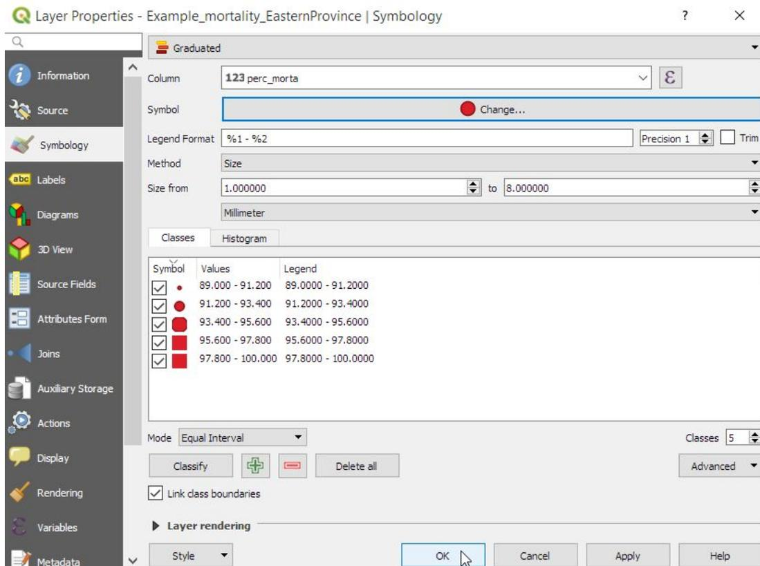
If you are not happy with the automated intervals you can change these either by changing the mode in which the intervals are generated from Equal Interval to another method, or you can edit the Values column manually.
